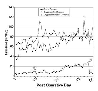
Fig 2. Measurements of arterial pressure, inlet oxygenator pressure, and pressure differential across oxygenator over the course of device support. The two oxygenator changes are marked by circled numbers adjacent to the pressure differential values.
